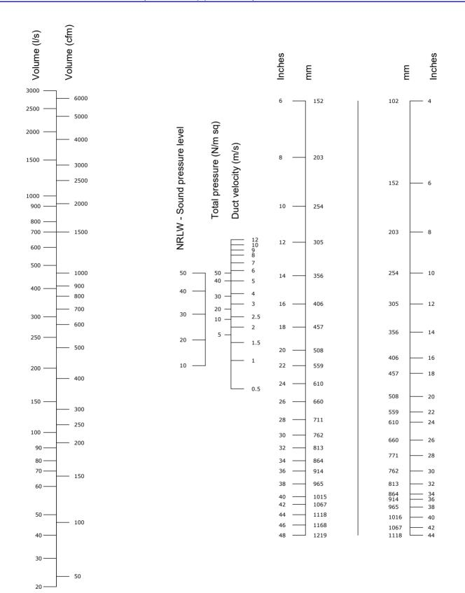
When using an SD grille for supply, refer to DD nomogram for figures. Sound power & pressure levels are based upon exhaust air with dampers fully open. Without dampers subtract 2dB and multiply total pressure by 0.9.
