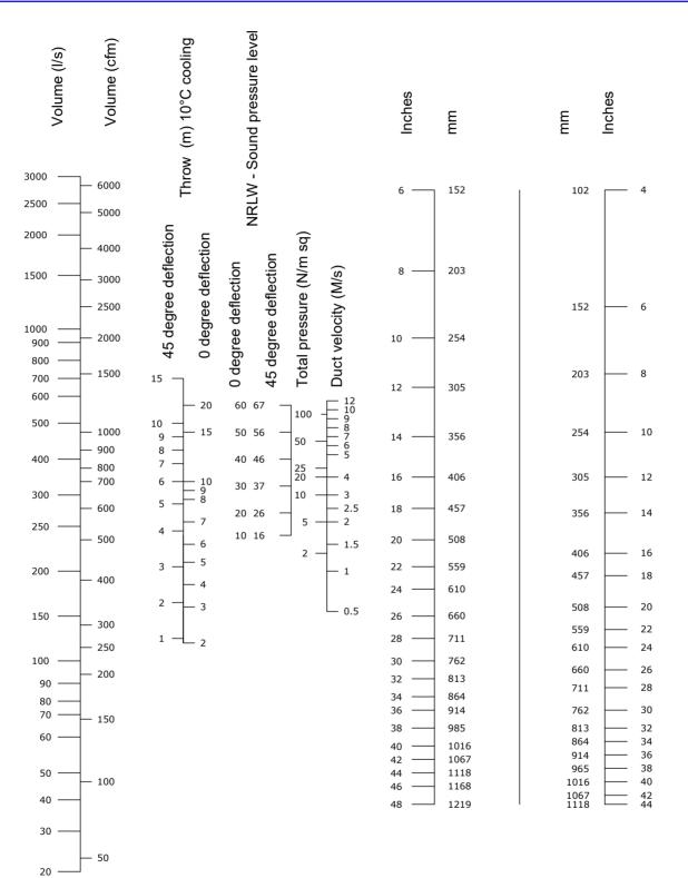
Throw values based on grilles mounted in sidewall not more than 1m below an unrestricted ceiling For grilles positioned more than 1m below an unrestricted ceiling, reduce throw values by 25%.
