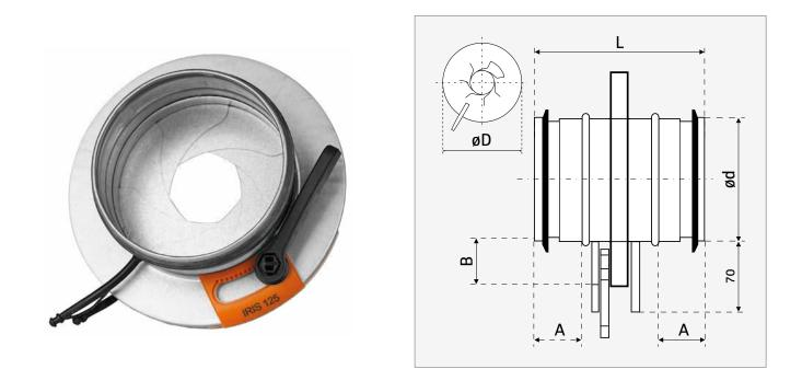
With IRIS damper, the intensity of air flow may be smoothly adjusted. Adjustment is done with a handle located on the damper which changes the diameter of the opening in the damping orifice. The damper is supplied with two endings which may be used to connect instruments measuring intensity of air flow. The damper is also supplied with a gasket, which tightens connection with the system.
