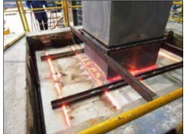
Series 100 fire damper during a horizontal fire test The test was stopped after 4 hours and 24 minutes because the 150mm thick concrete slabs themselves were failing. Damper leakage was actually decreasing at this stage.
